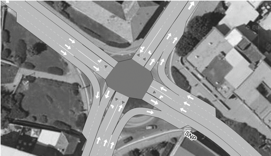
Fig. 6. Designed transport model with traffic-light controlled junction
