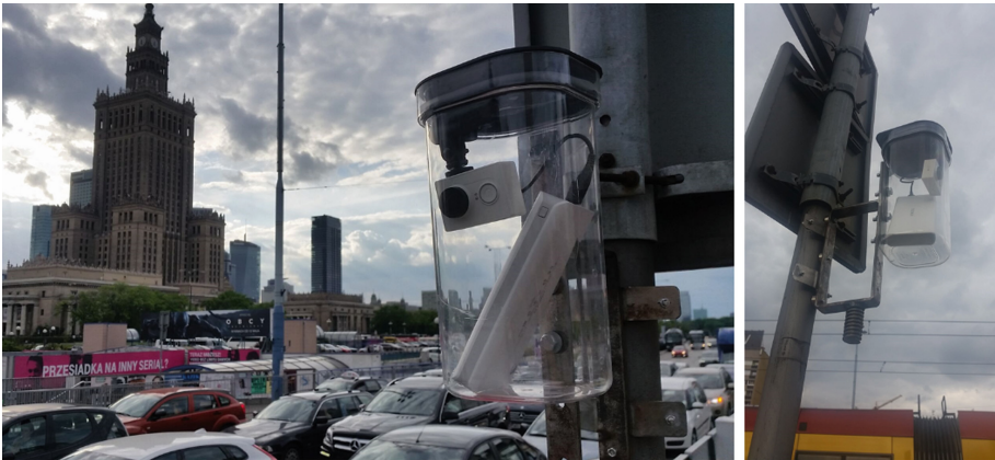
Fig. 5. Fixing a measurement kit to a road sign pole with neodymium magnets within a traffic measurement section in Warsaw (Source: [17])
