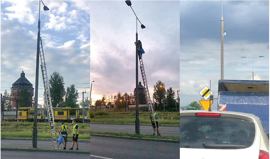
Fig. 7. Mounting measurement equipment along Kamienna Street in Bydgoszcz using rope and ladder access (Source: [17])
