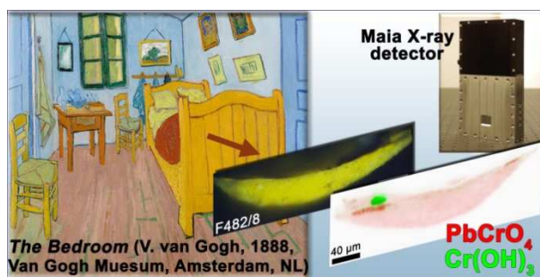
FIG. C-3. Adapted from: MONICO, L., et al., “Full spectral XANES imaging using the Maia detector array as a new tool for the study of the alteration process of chrome yellow pigments in paintings by Vincent van Gogh”, J. Anal. At. Spectrom. 30 (2015) 613–626.
