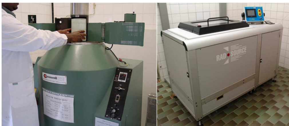
FIG. F-4. Gamma ray (left) or X-ray (right) irradiators are used for sterilization of male mosquitoes. (Photo: IAEA)
