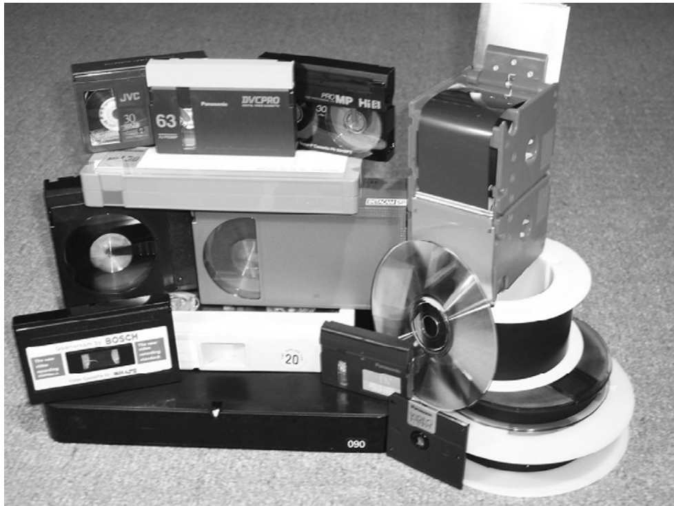
FIGURE 9.10 Audio and video recording stock is manufactured in a great variety of widths, thicknesses, and magnetic coatings depending on the purpose for which the tape is intended. The recording media today moves from magnetic tape to disc and on to solid-state media. From top down on the left: Mini-VHS, DVCPRO, Hi8, M-II, BetaMax, BetaSP, Quarter-cam, U-matic, DV. On the right: two-inch quad cart, two-inch quad open reel, EIAJ 1/2-inch, Type "C" one-inch. In front of the reels, a DVD and 1/2-inch floppy.
