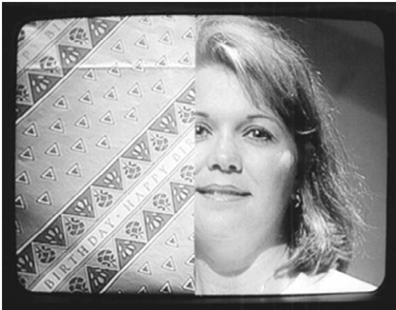
FIGURE 5.17 A wipe appears as one image is replaced by another with a straight line separating the two images. A wide number of different patterns separating the two images also may be used.
