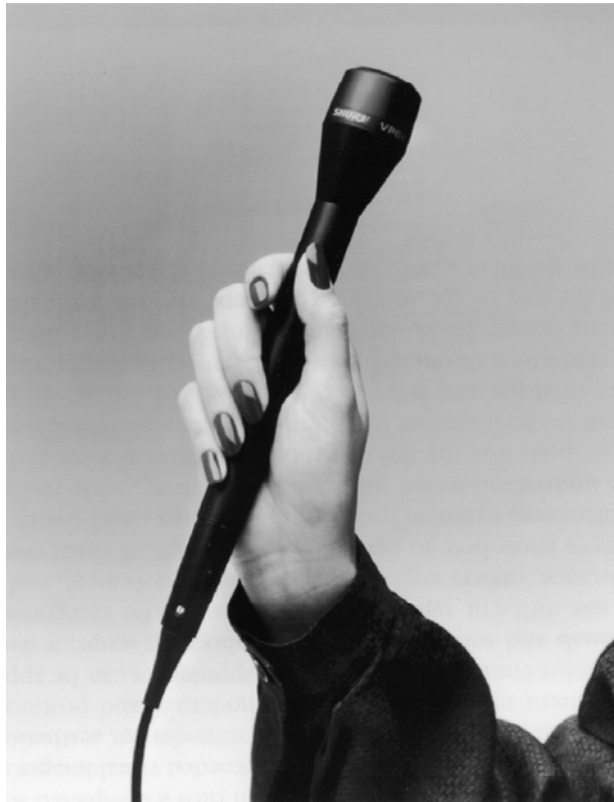
FIGURE 6.4 Hand microphones also may be mounted on a desk stand, floor stand, or boom, but they must be designed to fit comfortably in the hand with reasonable sensitivity. (Courtesy of Shure.)
