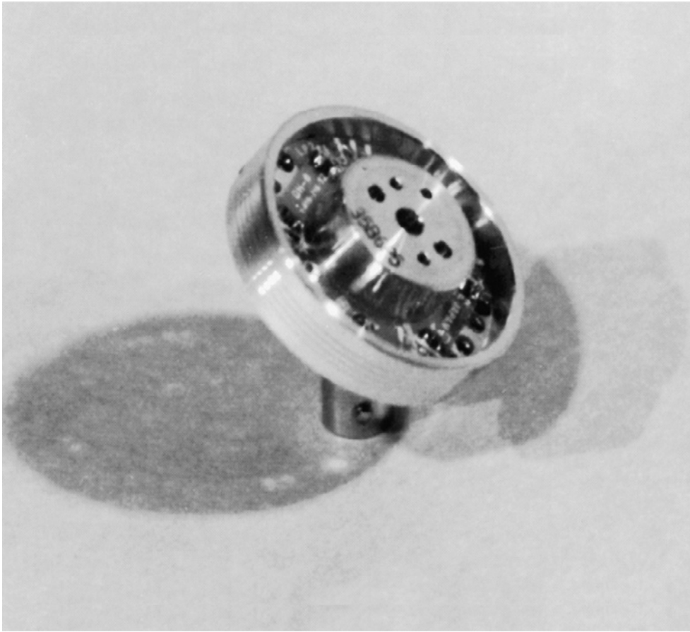
FIGURE 9.8 The video head of a helical recorder contains from two to eight different recording or erasing heads depending on the complexity of the format.
