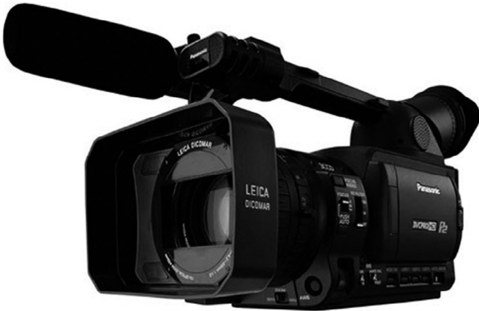
FIGURE 8.15 HDV cameras usually use built-in miniDV tape decks or limited memory flash cards. The optics are superior to basic DV cameras but not as expensive or flexible as those used on HD or broadcast cameras. (Courtesy of Panasonic USA.)
