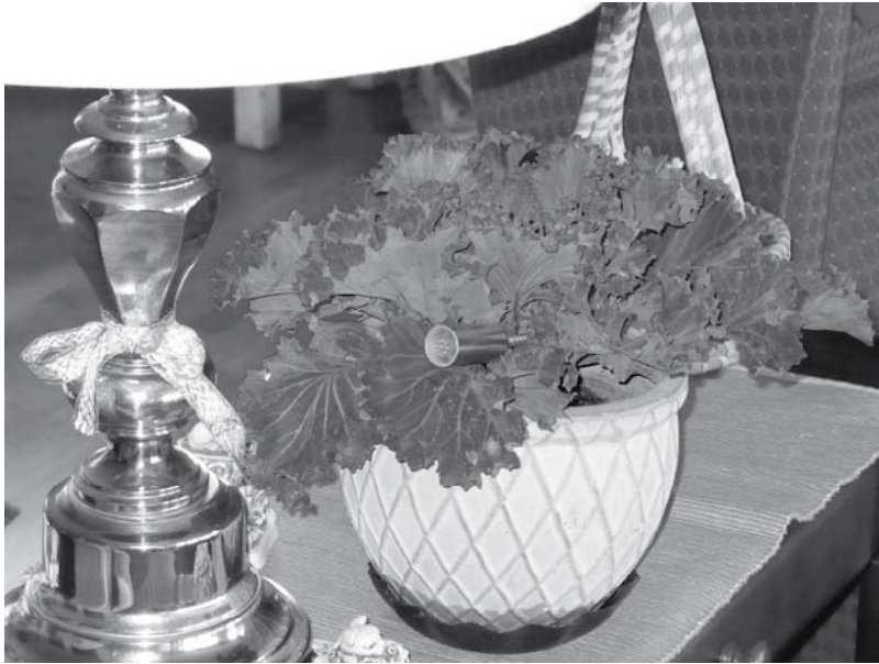
FIGURE 6.13 If the production requires off-camera mics, a microphone also can be concealed in a set piece or hand prop on a set near where the actors will be talking.
