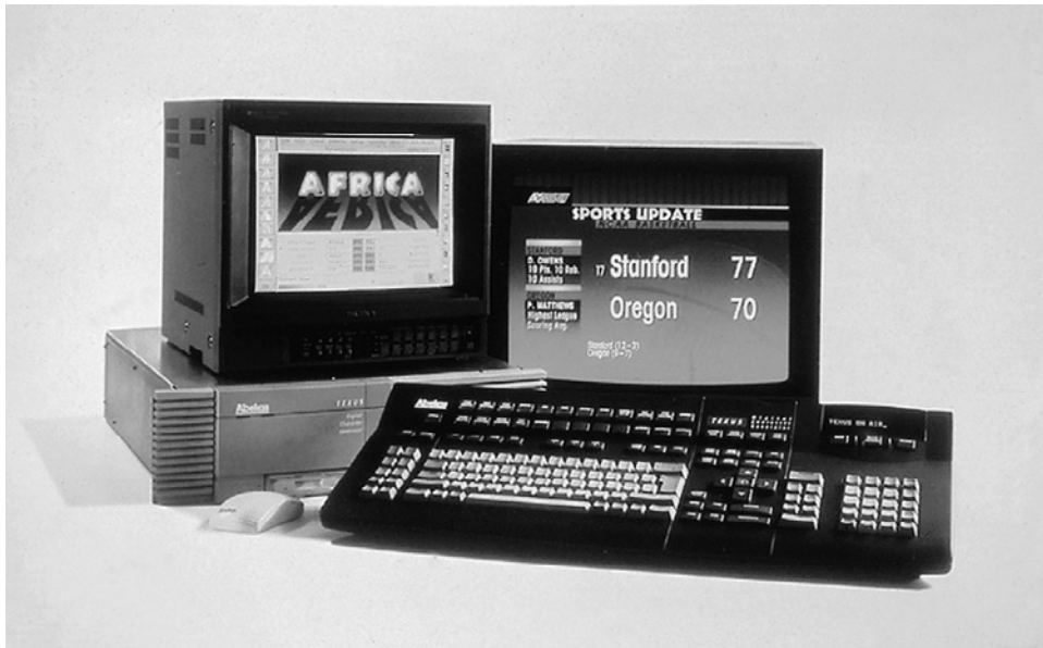
FIGURE 11.12 A character generator (CG) is a relatively simple computer graphics machine designed to create lines of type, including numbers, and simple color graphics backgrounds or lines of type to be keyed over other video frames. (Courtesy of Scitex Digital Video.)
