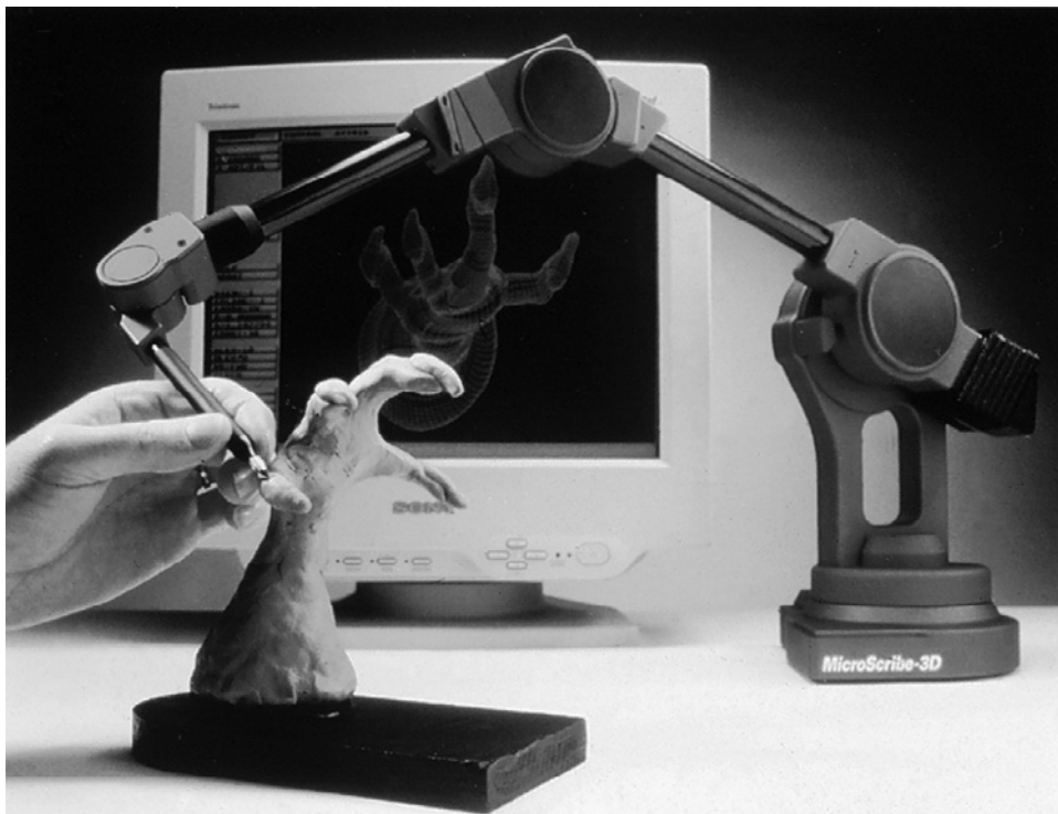
FIGURE 11.19 One of the methods of converting a solid object to a digital form is by tracing that form using a 3-D digitizer. The operator traces over all key surfaces of the object with a stylus until a full 3-D image has been transferred to a digital file. (Courtesy of Immersion Corporation.)
