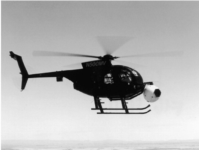
FIGURE 5.8 Among many other means of mounting either film or video cameras is the gyroscope mount, which can be mounted on an airplane, helicopter, or any moving vehicle. The stabilizing system provides a solid, smooth picture, and the operator inside the vehicle can pan, tilt, and zoom the camera as the shot requires.
