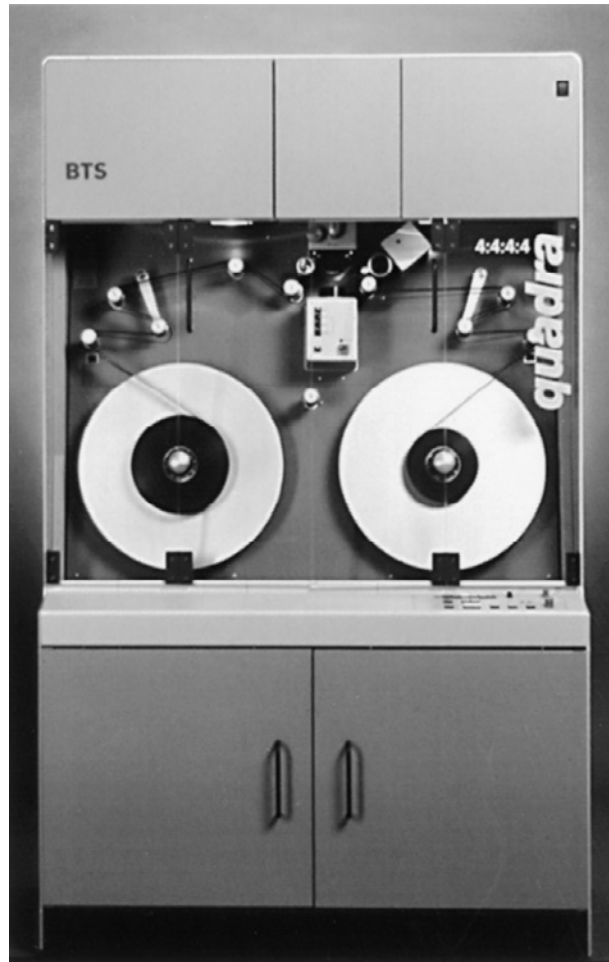
FIGURE 10.15 A CCD telecine film-to-digital conversion. Each film frame is scanned individually, allowing for color correction and filtering in real time as the film is converted to a digital signal. (Courtesy of Philips Broadcast Television Systems Company.)
