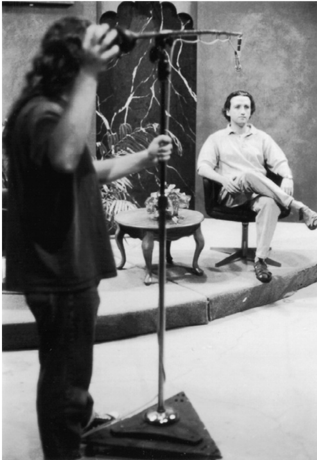
FIGURE 6.10 A giraffe microphone is a small boom generally used to pick up the voice of one or two persons in fixed locations.
