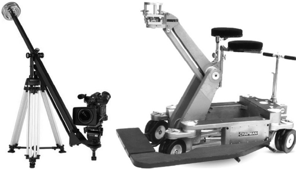
FIGURE 8.5 Dollies are constructed in a variety of shapes and sizes. These two are designed to be operated by hand rather than motorized. The dolly in the top photo is designed with the camera mounted in a yoke and with the operator and grip moving the camera and dolly as needed. The dolly in the bottom photo is designed for the camera operator to ride seated. (Courtesy of Miller Camera Support Equipment and Chapman/Leonard Studio Equipment.)
