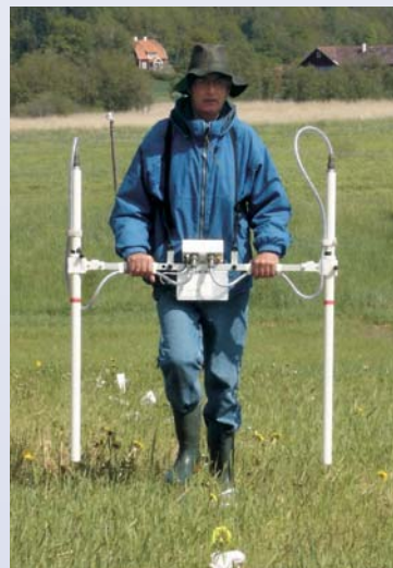
The Bartington Grad601-2 single axis, vertical component high stability fluxgate gradiometer system.
