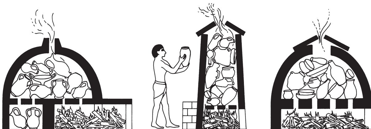
Pyrotechnology: the control of fire. Initially pottery was made in an open fire. The introduction of the potter's kiln meant higher temperatures could be achieved, also spurring on the development of metallurgy. (Left) Mesopotamian dome-shaped kiln of the early 4th millennium BC, built largely of clay, with an outer wall of stone or mud brick. (Center) Egyptian kiln of c. 3000 BC reconstructed from tomb paintings. The potter may have stood on the small platform to load the kiln. (Right) Greek kiln of c. 500 BC, reconstructed from scenes on Corinthian plaques: the extended fire opening probably improved combustion.
