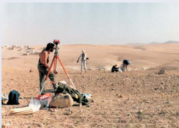
The survey and collecting team at Tell Halula, using a theodolite.
