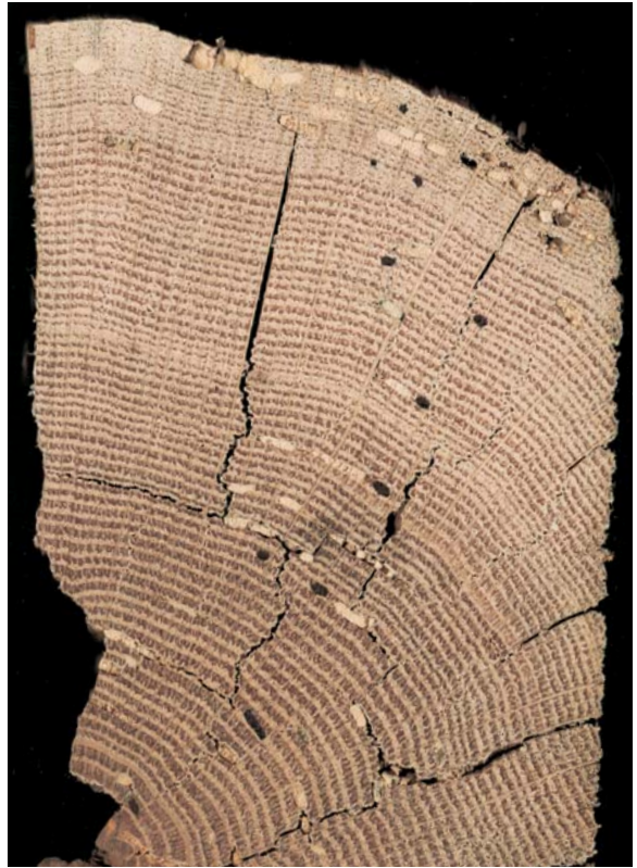
Section of an oak beam from the wall of a log cabin in Hanover, Pennsylvania, USA: the annual growth rings are clearly visible, and since this sample contains complete sapwood (top of image), a precise felling date of 1850/1 can be established.
