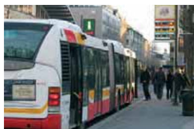
Low floor vehicles with 4 wide doors reduces stop time in Jönköping.
