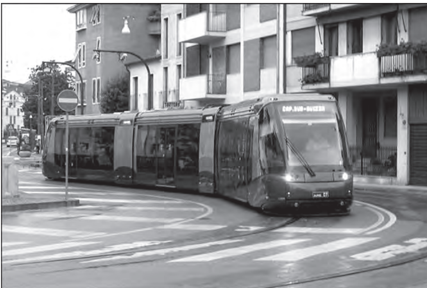
Figure 4.19 Translohr rubber-tyred single-guide rail vehicle (a bus rapid transit vehicle that is otherwise like a light rail transit vehicle) blurs modal distinctions in Padua, Italy
