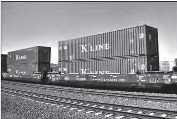
Figure 5.5 Double-stack container trains can be up to 1 mile (1.6km) long
