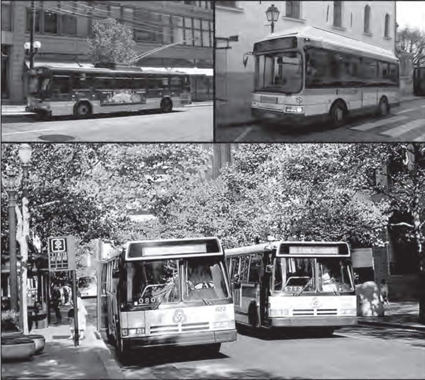
Figure 4.7 Electrified trolley bus in Seattle, Washington (top left); electrified mini-bus in Montmartre, Paris (top right); a properly done transit mall in Portland, Oregon, with lanes sufficient for boarding passengers as well as for passing buses (bottom)
