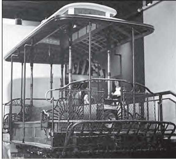
Figure 3.4 Historic cable car at the Smithsonian National Museum of American History: The front metalwork protruding at an angle was lowered in operation in order to act as a 'pedestrian catcher'
