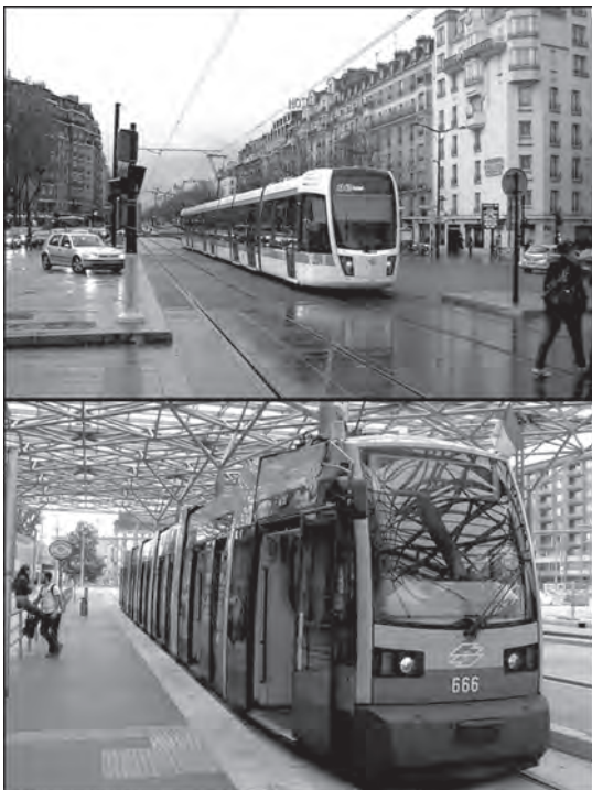
Figure 4.8 Modern light rail transit (LRT) on the T3 line in right of way (RoW) B in Paris crosses an intersection where traffic has been stopped by a transit priority signal control (top); Vienna's ultra-low floor LRT operates in RoW C and B (bottom)
